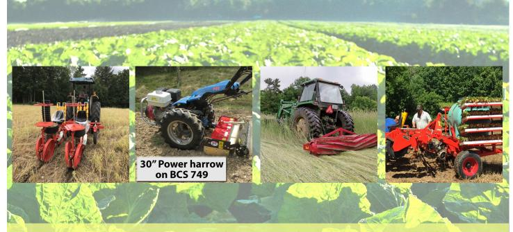
Featuring a two-wheel BCS tractor with various implements useful for vegetable growers, a no-till transplanter for planting and optimizing soil health, and tarping and roller crimper techniques for terminating cover crops.
