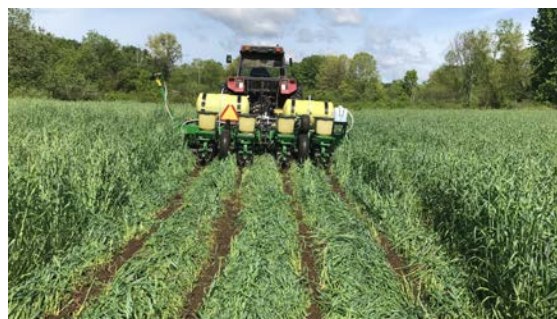
Planting green into a winter rye cover crop using a no-till planter with integrated cover crop rollers.
