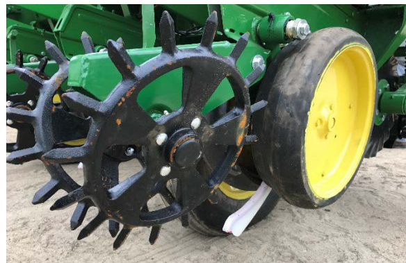
Spiked closing wheels help fracture sidewall compaction and assure the seed trench is fully closed in challenging soil conditions.
