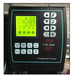
Monitor your ground speed. The planter is designed to plant at 3.5 - 5 mph. Do NOT exceed the maximum speed. This causes doubles and triples, as well as wear on the planter. Planting too slow can cause skips. The population monitor has a GPS based speedometer in the upper display. You can also use your tractor speedometer if you prefer, but the GPS speed sensor is used by the monitor to measure population.
