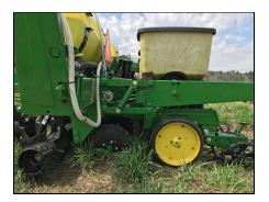
❑ Adjust the seed brush. On the side of the seed meter, you'll notice the seed size chart (at right) and adjustment t-handle. Move the handle to match the size seed you're planting. <u>Be gentle</u>! It's easy to pull the handle out of the meter. Size 3 is the same as the factory John Deere brush.
